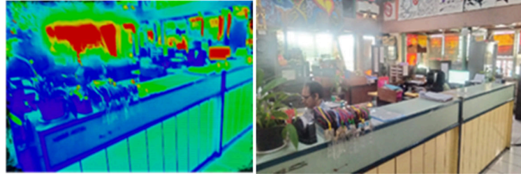
Figure 2 Thermal analysis in the Administration Room with a FLIR ONE camera and a regular digital camera
