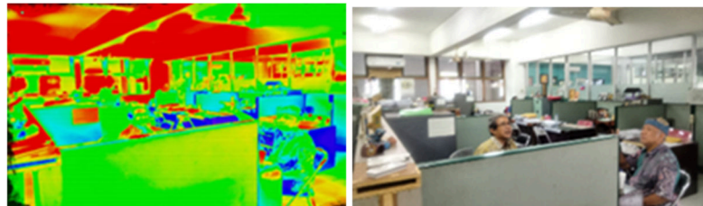
Figure 3 Thermal analysis in the Lecturer Room with a FLIR ONE camera and a regular digital camera
