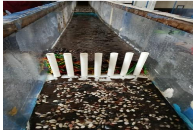
Gambar 3 Tampak Depan Sabo Dam Tipe Beam.
